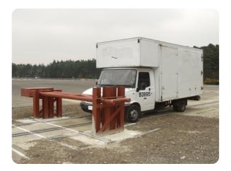
Gates | Rising Manufacturer:Multiple manufacturers (see specification) Standard Tested To: PAS 68:2007 Performance rating: V/3500[N1]/80/90:2.2/0.0
