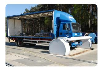
Gates | Retractable Manufacturer:ATG Access Standard Tested To: PAS 68:2007 Performance rating: V/7500[N3]/80/90:0/0.0
