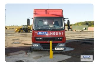
Bollards | Static Manufacturer:Safetyflex Barriers Standard Tested To: PAS 68:2007 Performance rating: V/7500[N2]/48/45:3.3/0.0
