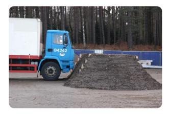
Perimeter Barriers | Vehicle Manufacturer:J & S Franklin Ltd Standard Tested To: PAS 68:2010 Performance rating: V/7500[N3]/80/90:2.5/0.0
