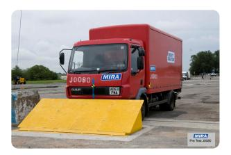
Blockers | Retractable Manufacturer:Security Solutions Northern Ltd Standard Tested To: PAS 68:2010 Performance rating: V/7500[N2]/48/90:0/0.0
