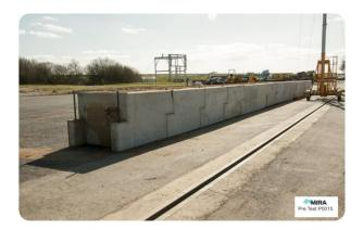
Perimeter Barriers | Modular Manufacturer:KarabloK UK Standard Tested To: IWA 14-1:2013 Performance rating: V/7200[N2A]/64/90:0.4
