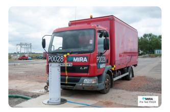
Bollards | Retractable Manufacturer:Swaraj Secutech Pvt. Ltd Standard Tested To: IWA 14-1:2013 Performance rating: V/7200[N2A]/80/90:0.8
