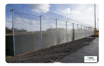
Perimeter Barriers | Pedestrian Manufacturer:Multiple manufacturers (see specification) Standard Tested To: IWA 14-1:2013 Performance rating: V/7200[N2A]/64/90:6.9
