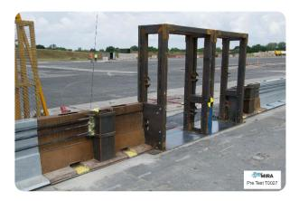
Portals | Pedestrian **Manufacturer:**Multiple manufacturers (see specification) **Standard Tested To:** IWA 14-1:2013 **Performance rating:** V/7200[N2A]/48/90:0
