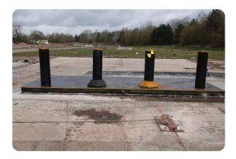
Bollards | Sliding Manufacturer:Heald Ltd Standard Tested To: IWA 14-1:2013 Performance rating: V/7200[N2A]/80/90:3.2
