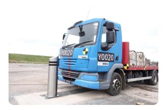
Bollards | Retractable Manufacturer:Safetyflex Barriers Standard Tested To: IWA 14-1:2013 Performance rating: V/7200[N2A]/80/90:3.1
