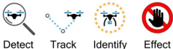
**Detect, Track, Identify, Effect (DTIE) Technology** that can be used to provide security personnel with the timely and accurate information they require to enable a proportionate and effective response which includes using a technical effect to prevent the UAV from completing its intended activity.
