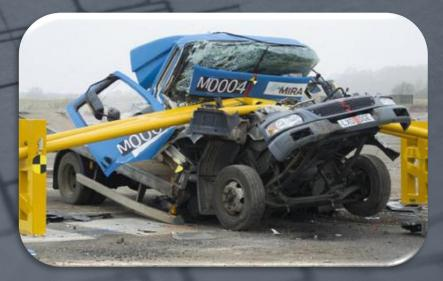
Repeatability is not easily achieved due to subtle changes in these parameters between tests. It is known that nuances around the vehicle construction are a factor on the performance of VSBs although tolerances in the standards reduce this to a pragmatic level.
