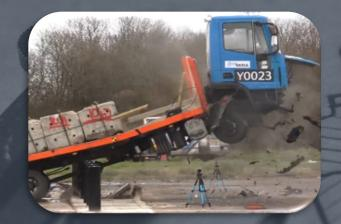
A VSB is a product designed to prevent vehicle access. It has undergone testing at an independent and accredited test house, to a recognised **vehicle impact test** standard and achieved a performance rating in accordance with that standard. The test, which is often destructive, demonstrates the VSB performance in reality, against a specified vehicle, speed and impact angle.
