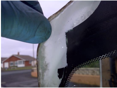
Figure 1: Edge delamination in car windscreen
