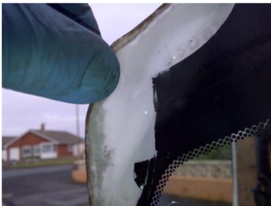
Figure 1: Edge delamination in car windscreen
