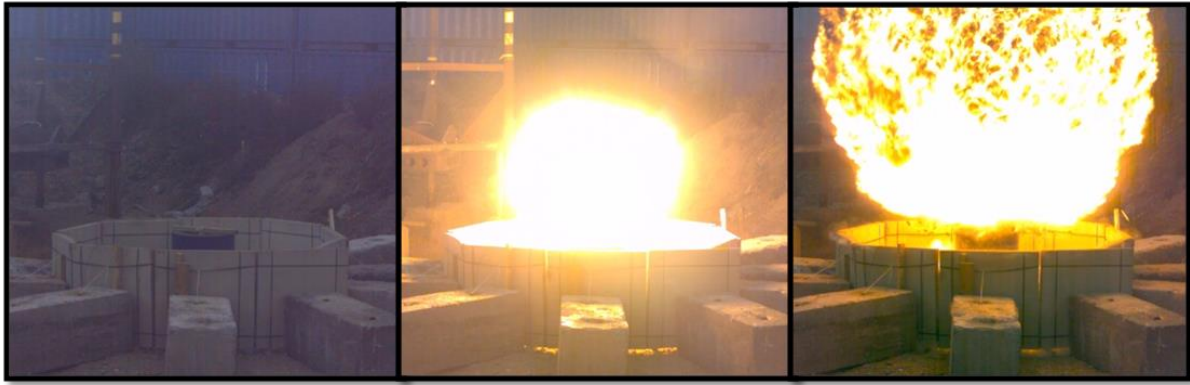
Figure 1: The developing fireball from a detonation within a blast-resistant litter bin
