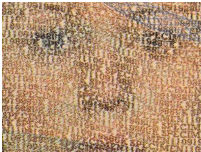
Example of LetterScreen on the observations page of the 2010 UK passport
