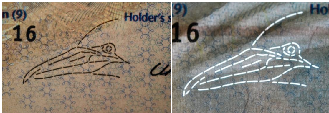
Two photos of DestriPerf® on the biodata page of the UK passport first issued in 2006 – the one on the left is face on, the one the right is using transmitted light
