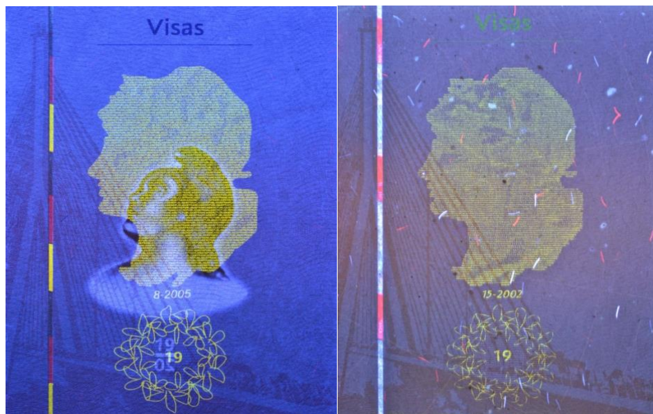
Counterfeit watermark (left), viewed with UV light. A genuine watermark should not fluoresce (right) – see also the image on page 7
