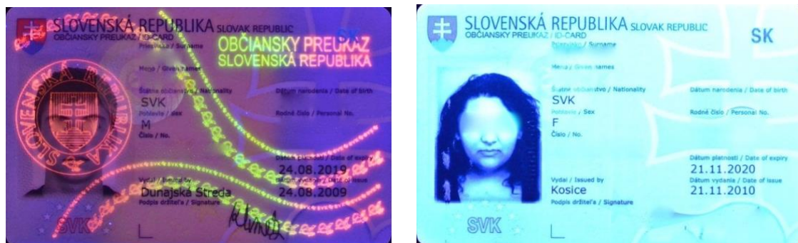
Examples of a genuine (left) and counterfeit (right) Slovakian identity card to show fluorescing of counterfeit substrate
