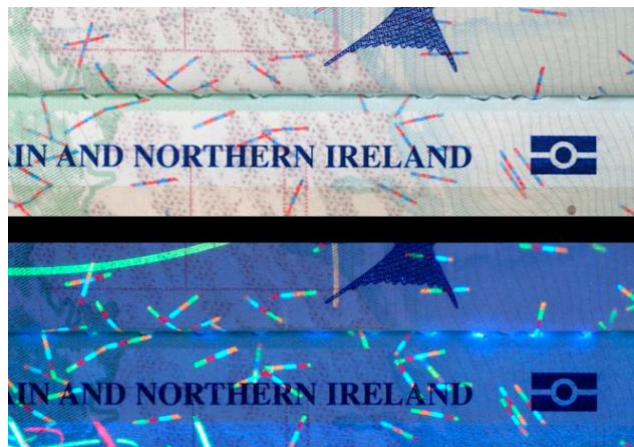
Security fibres under normal and UV light source in the UK passport first issued in 2010
