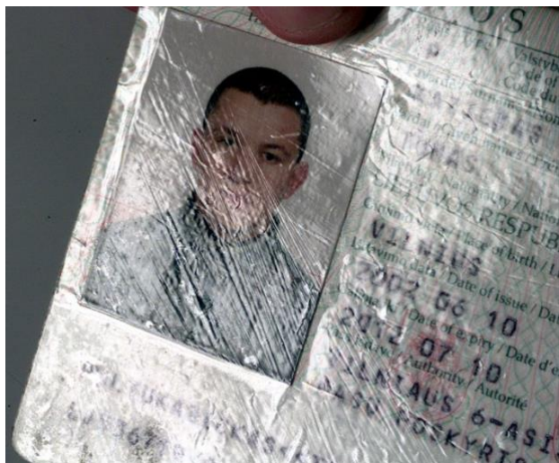
Damage to the laminate from the lifted laminate method seen under oblique light
