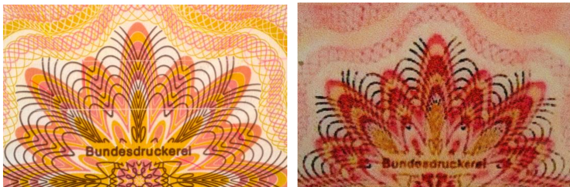
Examples of background printing on a genuine (left) and counterfeit (right) German identity card
