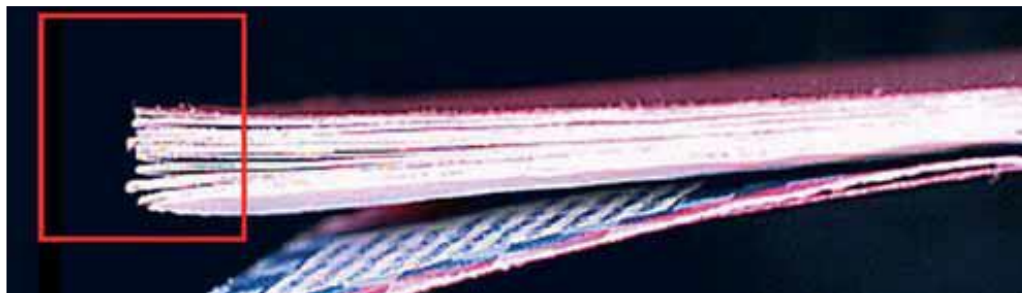
Photo shows poor alignment of pages when passport is closed
