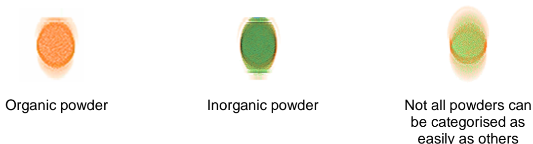
Figure 5: Example X-ray images of plastic pots containing different powders (viewed as if looking down through the container)
